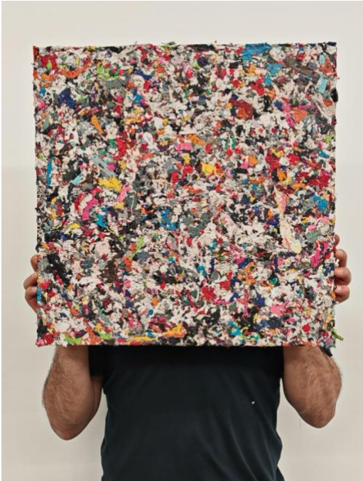
Image 4: Turning shredded textile waste into insulation material to be used in construction industry. Courtesy of KNOF.
